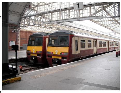
time class 320 trains had a top speed of 75mph which was too low for the new route and so they were largely superseded by the faster class 334 trains which had a top speed of 90mph. Subsequent modifications raised the top speed of class 320 trains to 90mph. See photo above.
