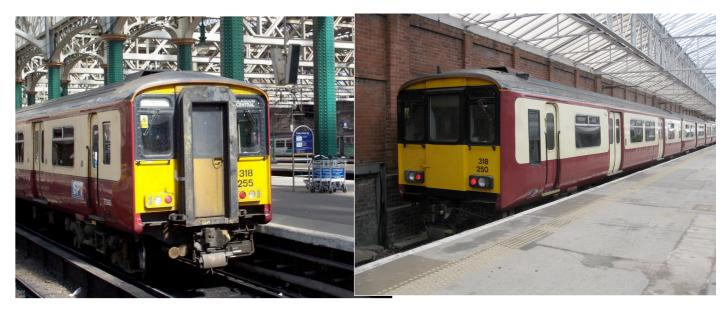
underwent a refurbishment which included the removal of the inter-unit gangway connection; this considerably altered their external appearance when viewed head-on, as can be seen from the photos above. They can often be seen running in tandem with Class 320 sets.
